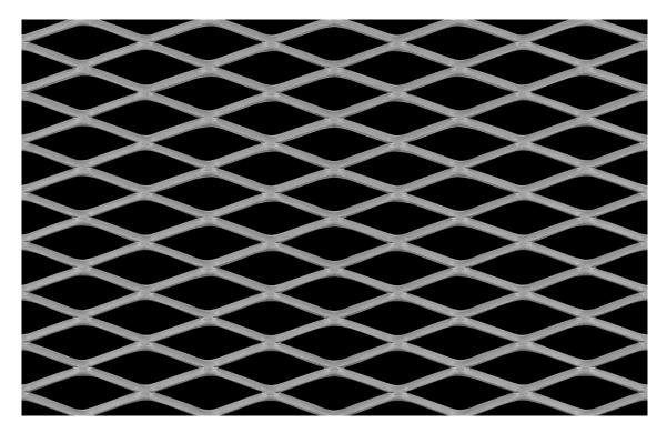
LW Aperture:24.38mmStrand Width:2.06mmSW Aperture:7.87mmThickness:1.50mmWeight:4.07 kg / m2Open Area:66%
